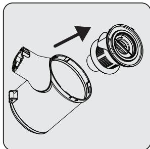
Pull EPA E10 and plastic filter holding from the EPA E10 handle.
