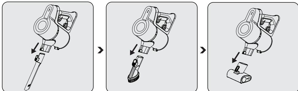
**Mini turbo brush (14):** Suitable for vacuuming floorings, stair steps, car interiors, sofas and seat, etc. It is also used for vacuuming pet hair on such surfaces.
